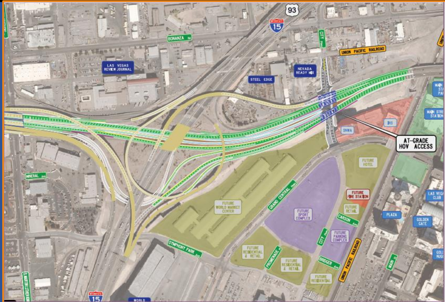
City Parkway Direct Access HOV Ramp Concept Sketch
